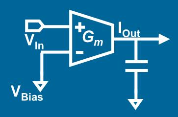
Extremely low transconductors or large capacitors are required for low frequency filters.
