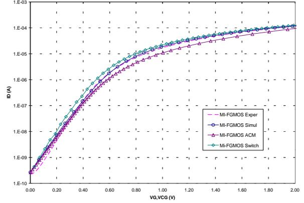
**Figure 6.**  $I_D$  vs.  $V_{CG}$  plots for experimental results, macromodel, analytical and transient simulations.
