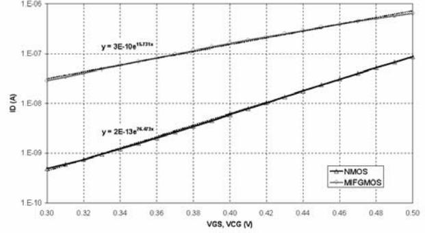
Figure 2.  $I_D$  vs.  $[V_{GS}, V_{CG}]$  in WI inversion,  $n=1.46$  and  $n_{CG}=2.46$ .
