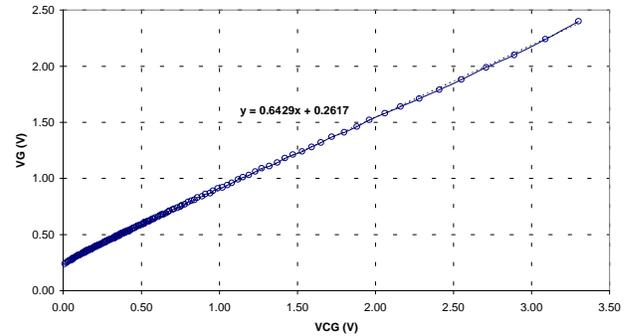
Figure 4.  $V_G$  vs.  $V_{CG}$ ,  $\alpha_{CG}=0.6429$  and  $V_{EQ}=0.2617$ .
