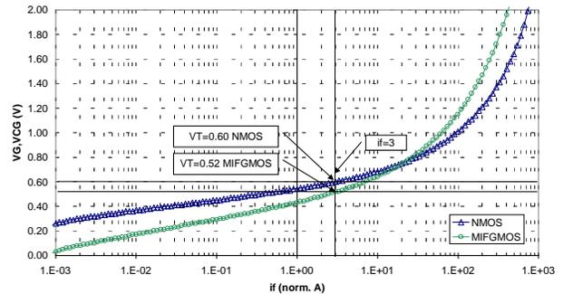
Figure 5.  $[V_G, V_{CG}]$  vs.  $i_f$ .  $V_T=0.6V$  and  $V_T^{CG}=0.52V$ .
