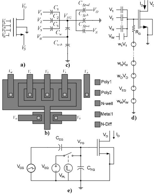
**Figure 1.** MI-FGMOS transistor. a) Symbolic representation. b) Layout representation. c) Equivalent capacitive circuit. d) Macromodel. e) Switched structure.
