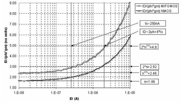
Figure 3.  $I_D / \phi_t g_{mg}$  vs.  $I_D$  for NMOS transistor and MI-FGMOS device,  $I_S \approx 250nA$ .
