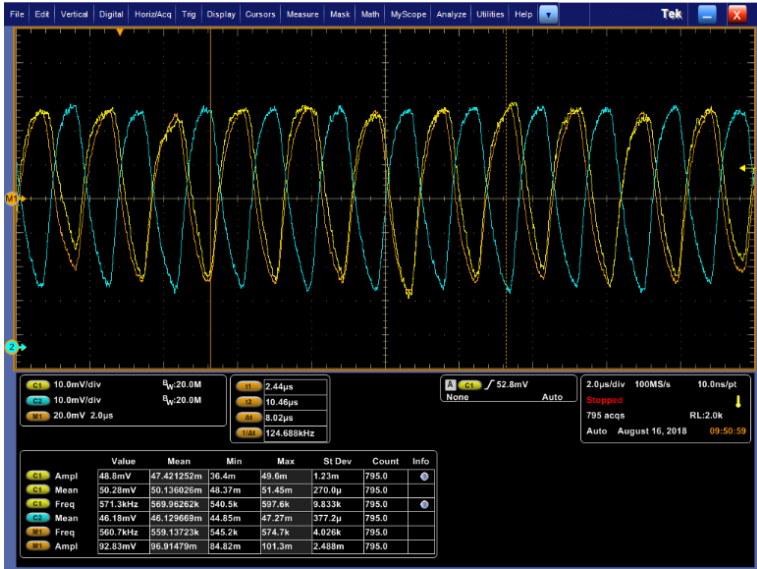
Figure 36 – INV RO oscillating at 80 mV
