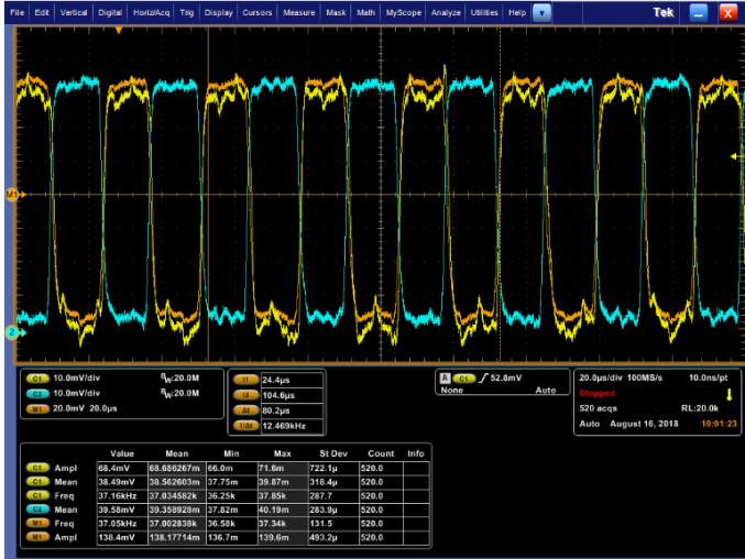
Figure 42 – STB RO oscillating at 80 mV
