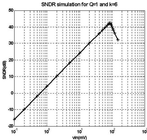
Figure 9 - SNDR simulation for Q=1 and a 6dB bump.
