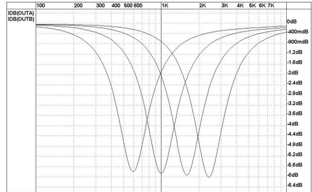
Figure 6 - Simulation results for center frequency programmability ( $Q = 1$ ).  $f_0 = 0.6, 1, 1.6,$  and  $2.6kHz$ ;  $V_{TUNE} = 40, 68, 113,$  and  $200mV$  respectively.
