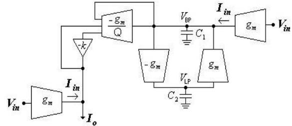
Figure 1 - Block diagram of the bump equalizer.
