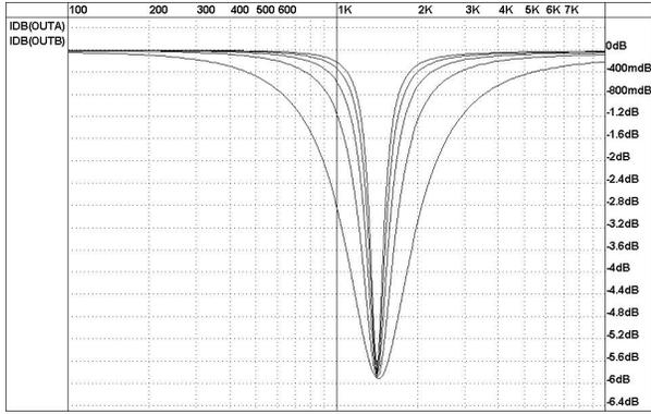
Figure 7 - Bandwidth programmability for Q=1, 2, 3, 4, and 5.
