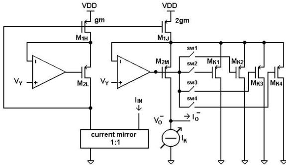
Figure 5 - Programmable current mirror (k-block)
