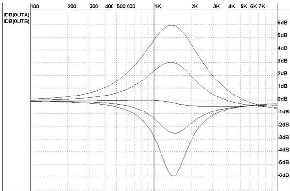
Figure 8 - Simulations results for bump/dip gain programmability k=6dB, 3dB, -3dB, -6dB.
