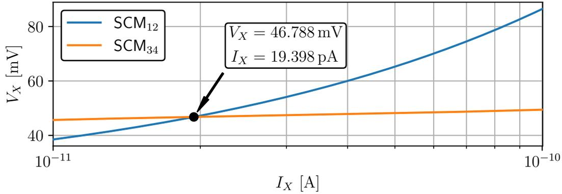
Figure 9 – Simulated curves for  $SCM_{12}$  and  $SCM_{34}$  after trimming. The highlighted point is the actual operating point.
