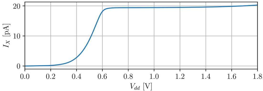
Figure 12 – Line regulation simulation for the designed SBCS core.
