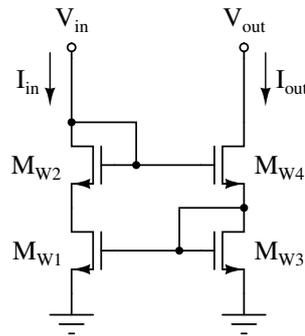
Figure 14 – Current reducing stage implemented with a four-transistor improved Wilson current mirror.
