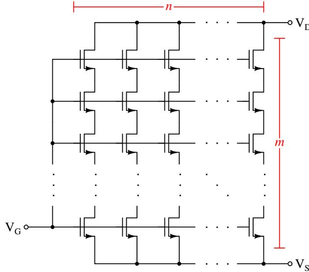
Figure 7 – Matrix of unit transistors.
