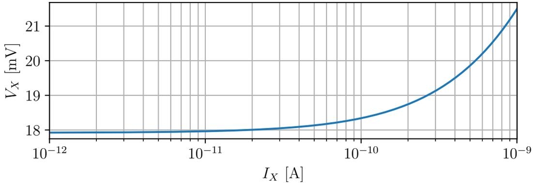
Figure 5 – Plot of eq. (3.6) with  $I_{sh} = 150$  nA,  $\alpha_{12} = 2$ ,  $S_2 = 0.01$  and  $\phi_t = 25.85$  mV.
