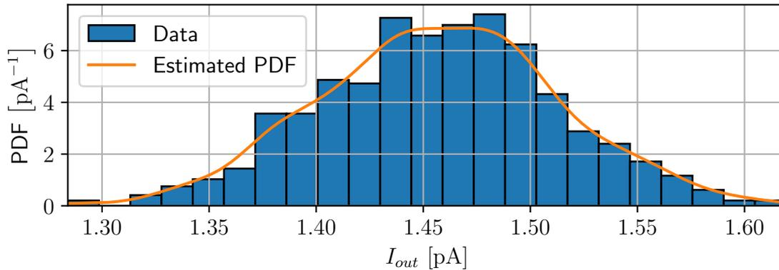
Figure 18 – Probability distribution of  $I_{out}$  due to component mismatch.
