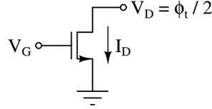
Figure 1 – Common-source configuration used for the extraction process.
