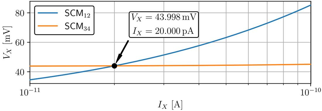
Figure 6 – Theoretical curves for  $SCM_{12}$  and  $SCM_{34}$ . The highlighted point is the intended operating point.
