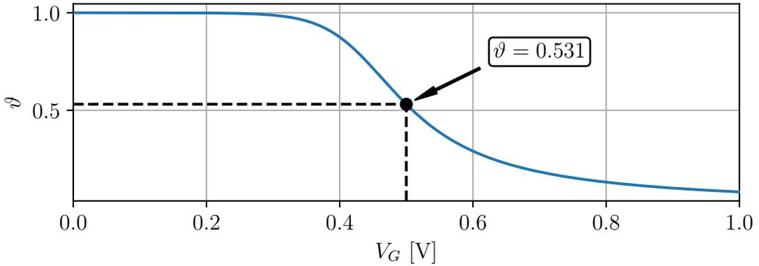
Figure 2 – Example plot of  $\vartheta \times V_G$  generated by the 3PM equations with  $I_s = 1 \mu\text{A}$ ,  $V_{T0} = 500 \text{ mV}$ ,  $n = 1.5$  and  $\phi_t = 25.85 \text{ mV}$ .
