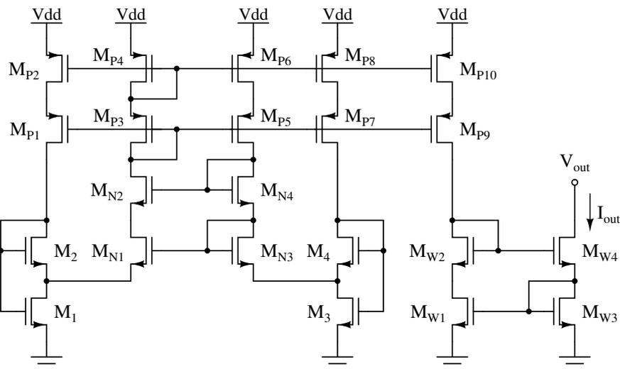
Figure 15 – Complete current source implemented by adding the current reducing stage from fig. 14 to the output of the SBCS core from fig. 11b.
