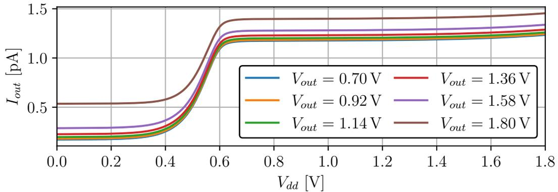
Figure 16 – Line regulation simulation for the full source for different output voltages.
