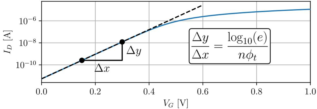
Figure 3 – Example plot of  $I_D \times V_G$  in log scale generated by the 3PM equations with  $I_s = 1 \mu\text{A}$ ,  $V_{T0} = 500 \text{ mV}$ ,  $n = 1.5$  and  $\phi_t = 25.85 \text{ mV}$ .
