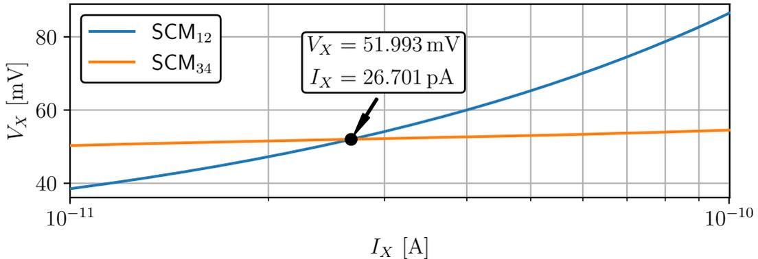
Figure 8 – Simulated curves for  $SCM_{12}$  and  $SCM_{34}$ . The highlighted point is the actual operating point.
