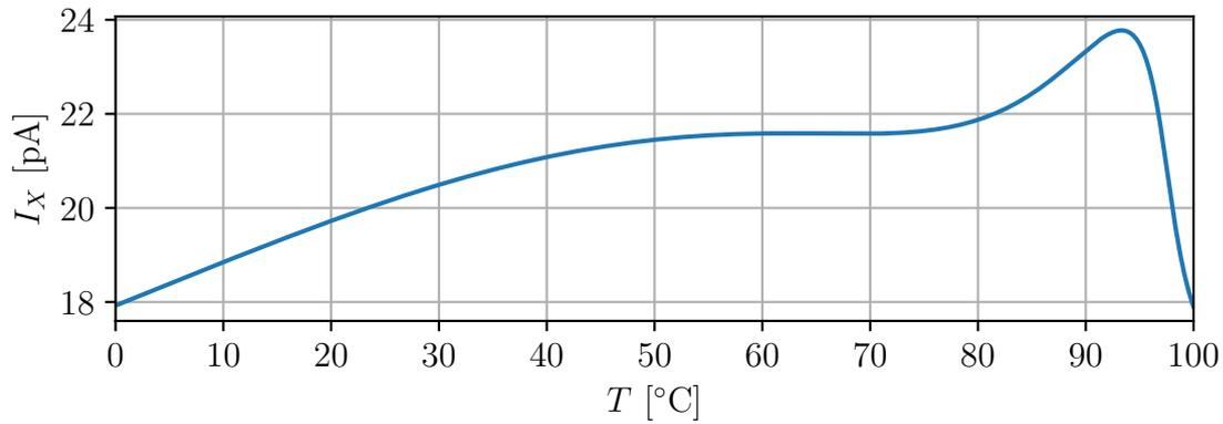
Figure 13 – Temperature simulation for the designed SBCS core.
