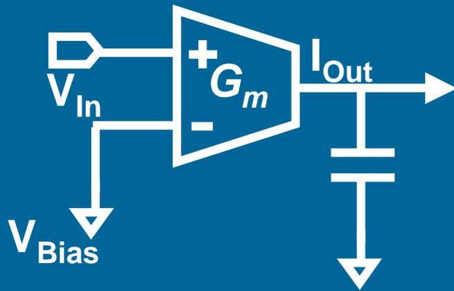
**Extremely low transconductors or large capacitors are required for low frequency filters.**
