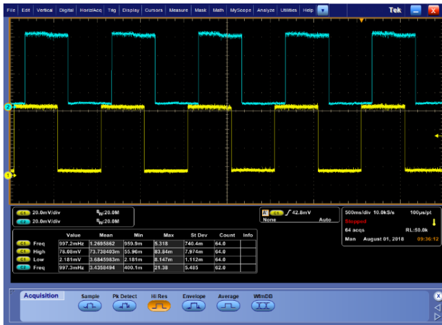
Figure 11. Output signals of the classical logic (upper wave) and ST logic (lower wave) frequency divider chains operating at 94mV
