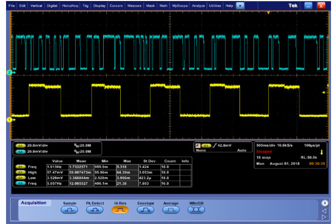
Figure 12. Output signals of both frequency divider chains at 76 mV of supply voltage. The classical logic (upper wave) does not operate properly, while the ST logic (lower wave) kept the signal of 1 Hz at 76 mV
