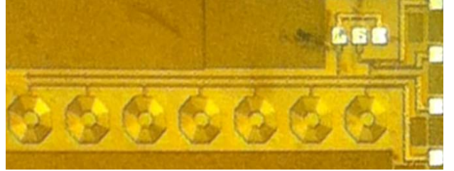
Figure 7. Micrograph of the seven-stage inductive ring oscillator in a 130 nm technology.
