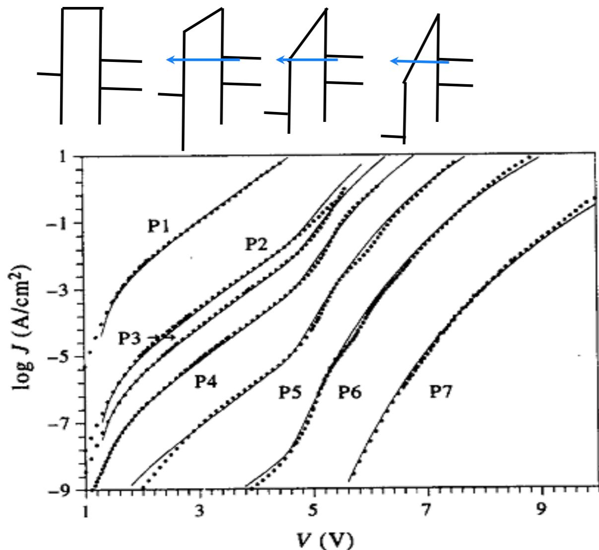
Fig. 1. Experimental and calculated—eqns (8) and (14)— $\log J$ - $V$  curves for all samples. Fitting oxide thicknesses are: P1—22.2 Å, P2—30.5 Å, P3—32.2 Å, P4—35.3 Å, P5—41.3 Å, P6—50.0 Å and P7—67.5 Å.
