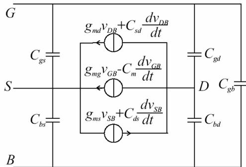
Fig. 3 Simplified small signal MOSFET model.
