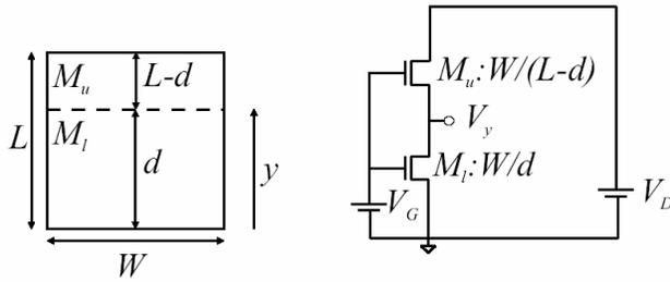
Fig. 2 Virtual cut of a transistor into two slices and its representation as a series association of transistors.
