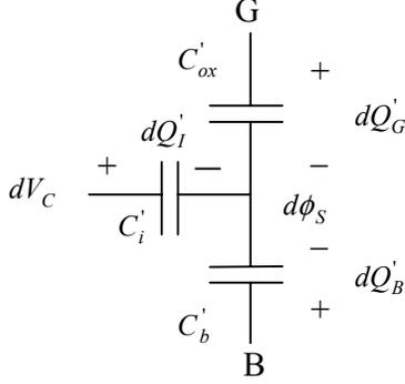
Fig. 1: Small-signal model for the three-terminal MOSFET
