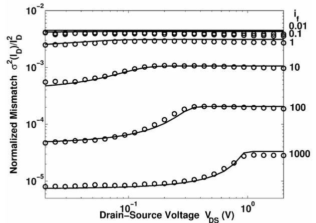
Fig. 5 Normalized mismatch of  $3\mu\text{m}/2\mu\text{m}$  ( $W/L$ ) n-channel MOSFETs of a TSMC  $0.35\mu\text{m}$  process, from linear (20mV) to saturation (2V) region, under a wide range of inversion levels ( $i_f$  is defined in Table II). Circles represent measurements while solid lines represent the mismatch model [10], [20].
