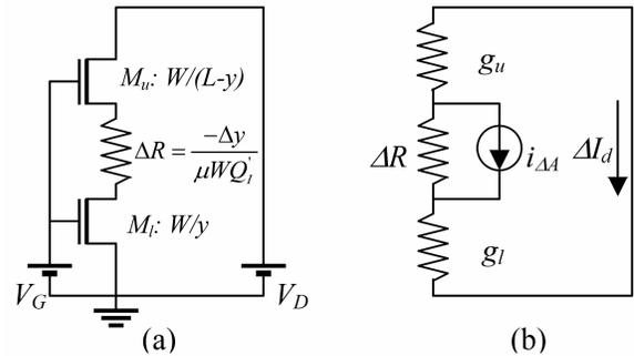
Fig. 4 Splitting of a transistor into three series elements: (a) transistor equivalent circuit and (b) small-signal equivalent circuit.
