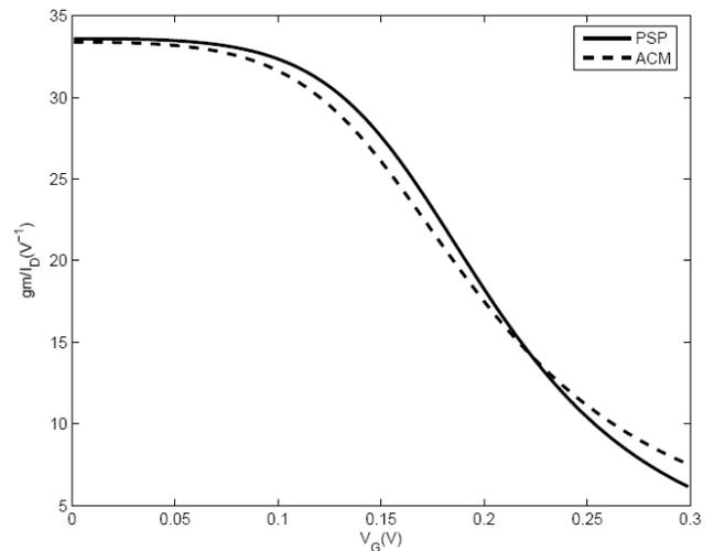
Fig. 7 Transconductance-to-current characteristic of an n-MOS transistor for  $V_{DS}=1$  mV. The PSP curve was used to determine both the threshold voltage and the sheet specific current.
