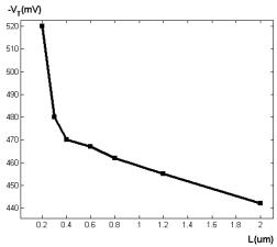
Fig.4. Threshold voltage vs. channel-length for a 0.18μm CMOS technology
