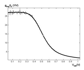
Fig.3. Transconductance-to-current ratio for  $V_{DB}=13 mV \cong \phi_{l'}/2$  and  $V_{SB}=0$ . Dotted line: measured  $g_{mg}/I_{D}$ ; solid line: filtered  $g_{mg}/I_{D}$ ; circle:  $g_{mg}/I_{D}=0.5310(g_{mg}/I_{D})_{max}$ .  $L_{m}=0.2~\mu m$  (mask channel length),  $W_{m}=20~\mu m$  (mask channel width). TSMC - 0.18  $\mu m$  technology.
