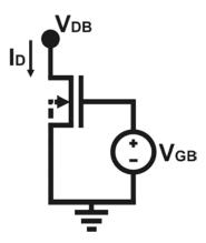
Fig.1: Circuit configuration for measuring the commonsource characteristics
