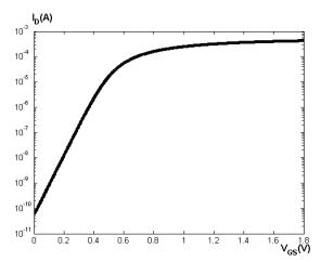
Fig.2. Drain current vs. gate voltage for  $V_{DB}=13$  mV  $\cong \phi_{t}/2$  and  $V_{SB}=0$ .  $L_{m}=0.2$   $\mu m$  (mask channel length),  $W_{m}=20$   $\mu m$  (mask channel width). TSMC - 0.18  $\mu m$  technology.
